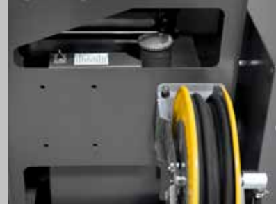
Emulsion spray system
